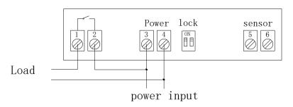
Load and temperature control use the different power
