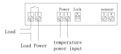
Terminals 1 and 2: The output of cooling and heating.
